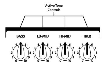
**BASS** controls the "weight" of the sound (50-150Hz). Many steel guitar players increase the bass somewhat to add fullness and compensate for the treble pickups used in typical pedal steels. The Steelaire has the headroom and speaker capacity to accept a substantial bass boost without "bottoming out".
