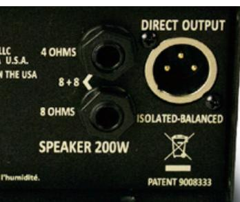
**CAUTION:** The Pro Block can provide enough power to blow many popular speakers. For safer results, use the MASTER to select a wattage limit that is reasonable for the speaker being used.
